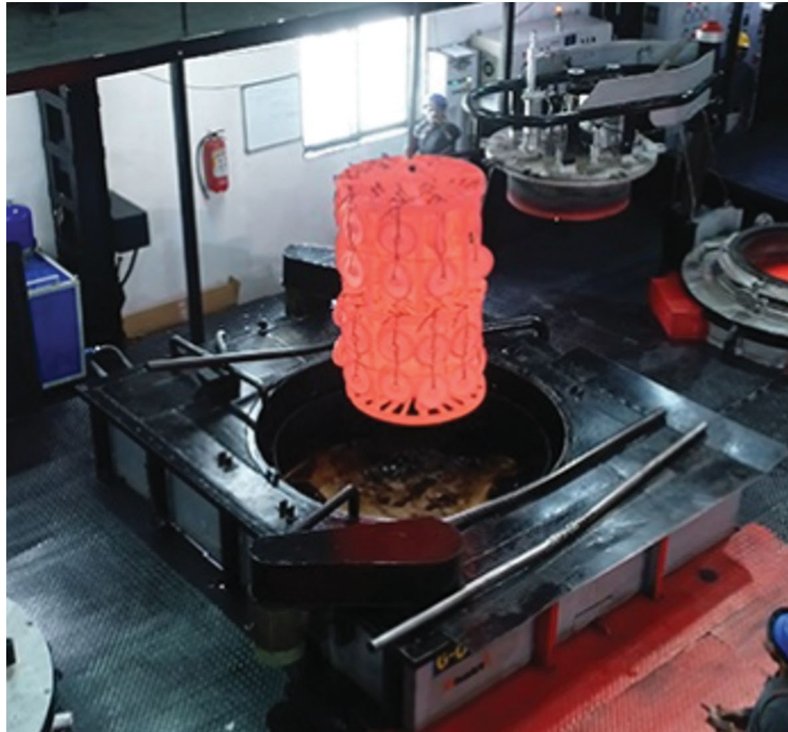
Part being immersed into oil quench tank, Shakti Heat Treaters
