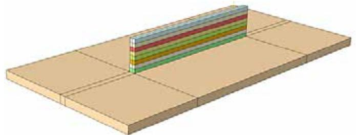
Figure 2: Finite-element model of build plate with color-coded welds.
