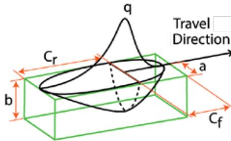
Figure 1: Goldak double ellipsoid parameters for flux distribution.
