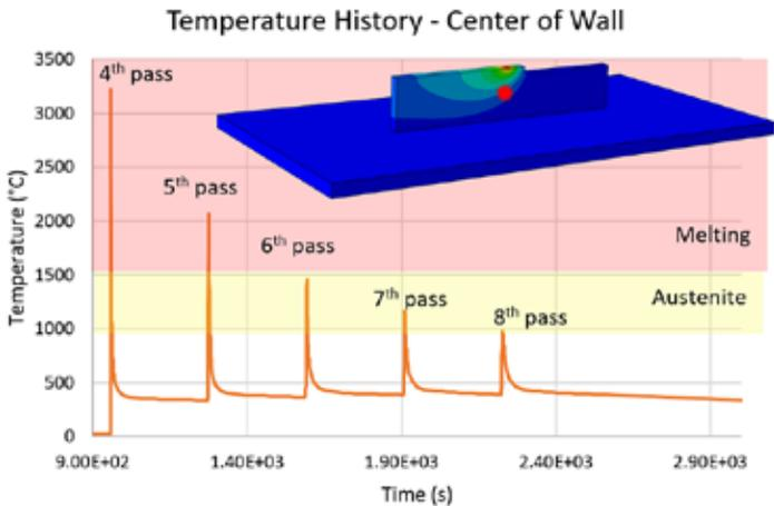
Figure 5: Temperature history of a point at the center of the build wall.
