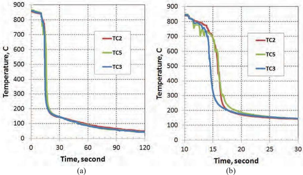
Figure 8 (a) Data for Quenching in Still Water - Test #4, and
