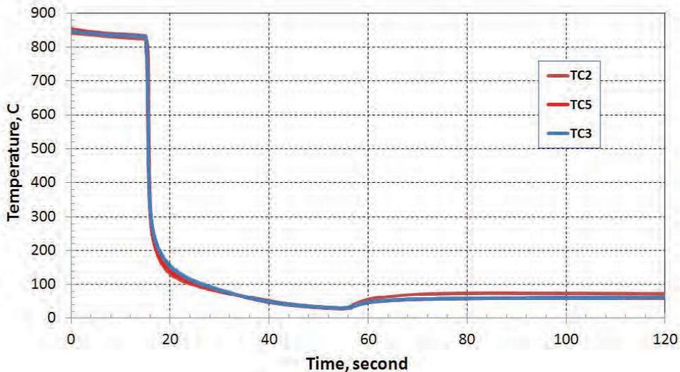
Figure 6 Quenching and Air Cooling Data for Test #2.
