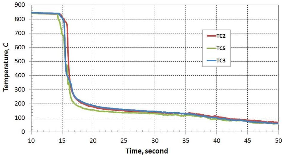
Figure 7 Data for Agitated Water Quench - Test #3.
