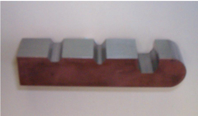
Figure 3:Machined Test Coupon Prior to Heat Treatment, showing Copper Masking for directional Carburization
