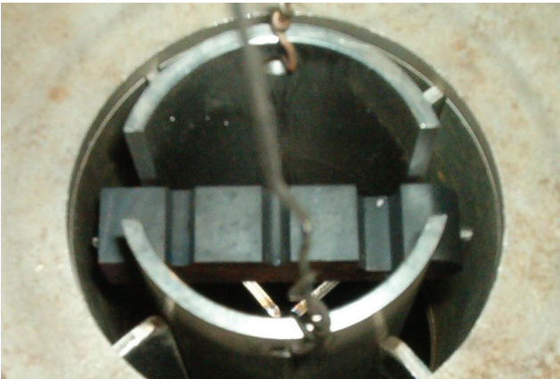
Figure 4: Triple Notched Test Bar in Intensive Quenching Heat Treating Fixture
