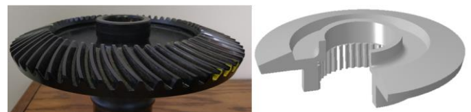
Figure 8: Bevel gear (left) and corresponding simplified CAD model (right) used for heat treat model.
