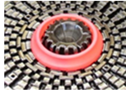
Figure 6: Hot bearing ring on lower die of the press quench machine just prior to quenching.
