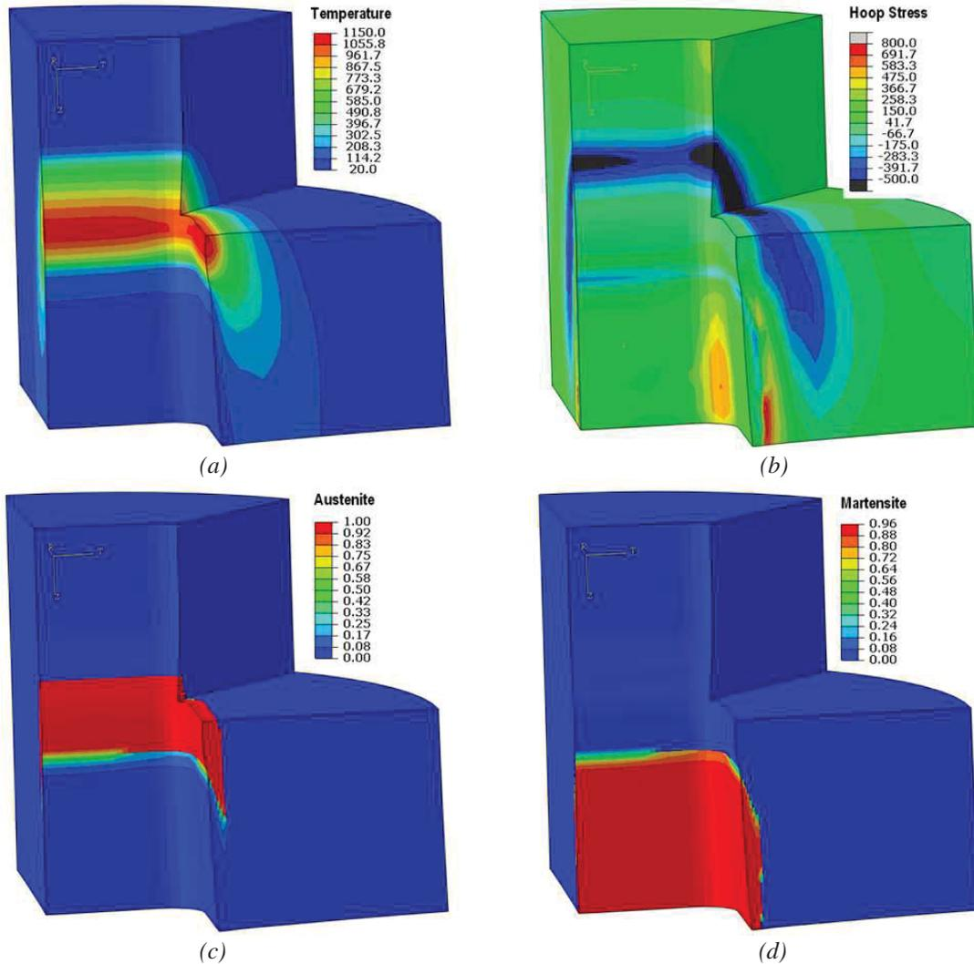
Figure 2: (a) Temperature, (b) hoop stress, (c) austenite, and (d) martensite distribution at 136.6 second during induction hardening process.
