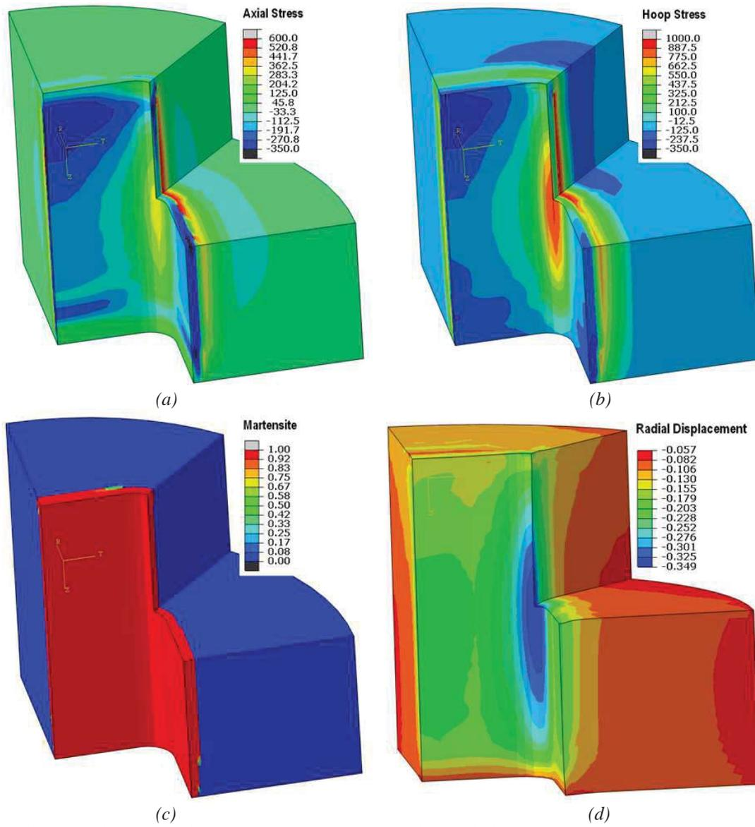
Figure 3: (a) Axial stress, (b) hoop stress, (c) martensite, and (d) radial displacement distributions at the end of induction hardening process.
