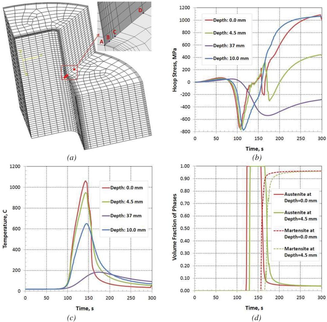
Figure 4: Evolution of temperature, hoop stress, and phase transformation during induction hardening process.
