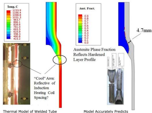
Thermal Model of Welded Tube induction heating is Calibrated to Physical Observation
