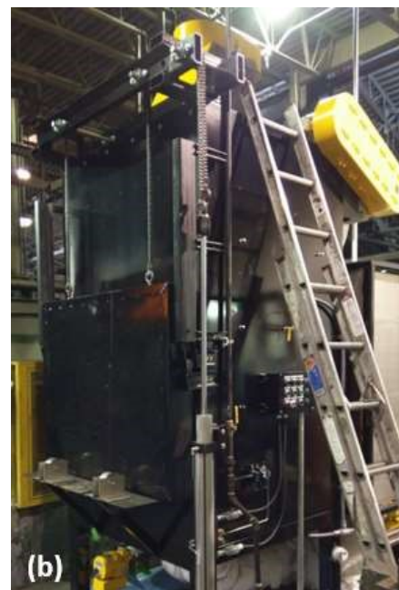
Figure 8. DCGQ equipment prototype. (a) HMI control panel, and (b) Front door of quenching chamber.
