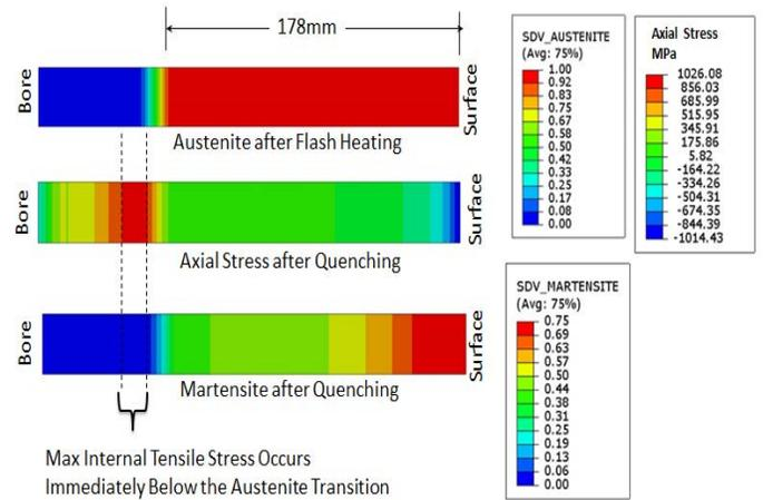
Figure 7: Composite contour plot showing flash heated austenitizing depth relative to the post quenching axial stress and martensite phase fraction profiles for the roll austenitized to 178mm depth.
